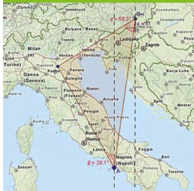
FIG.13 Triangle with measured angles
